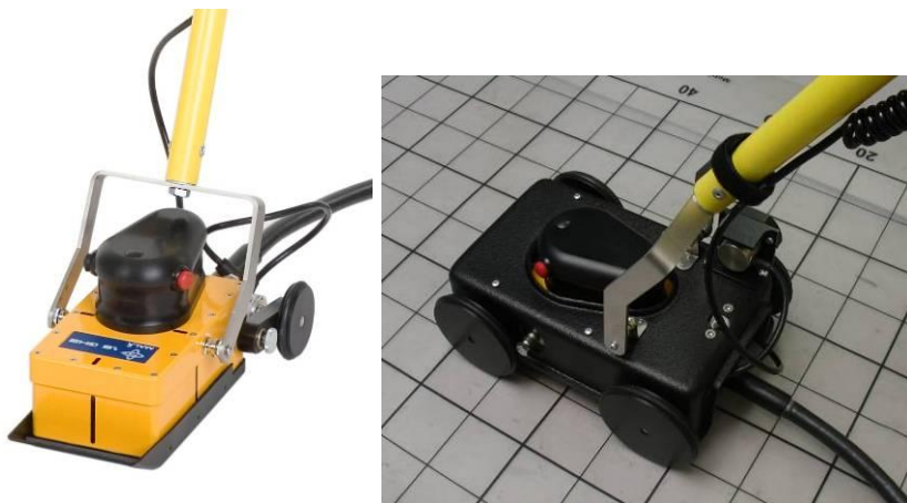
Figure 12.7 Mounting of the extension handle.
