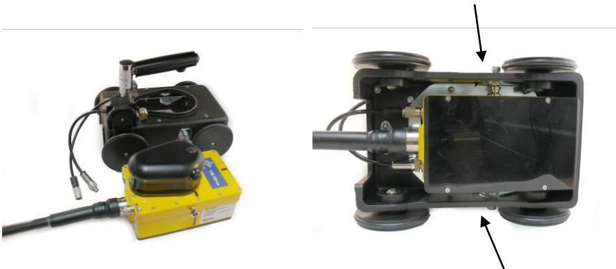
Figure 12.3 Mounting the HF antenna in the HF cart. The antenna is attached to the cart on two sides, see the arrows.
