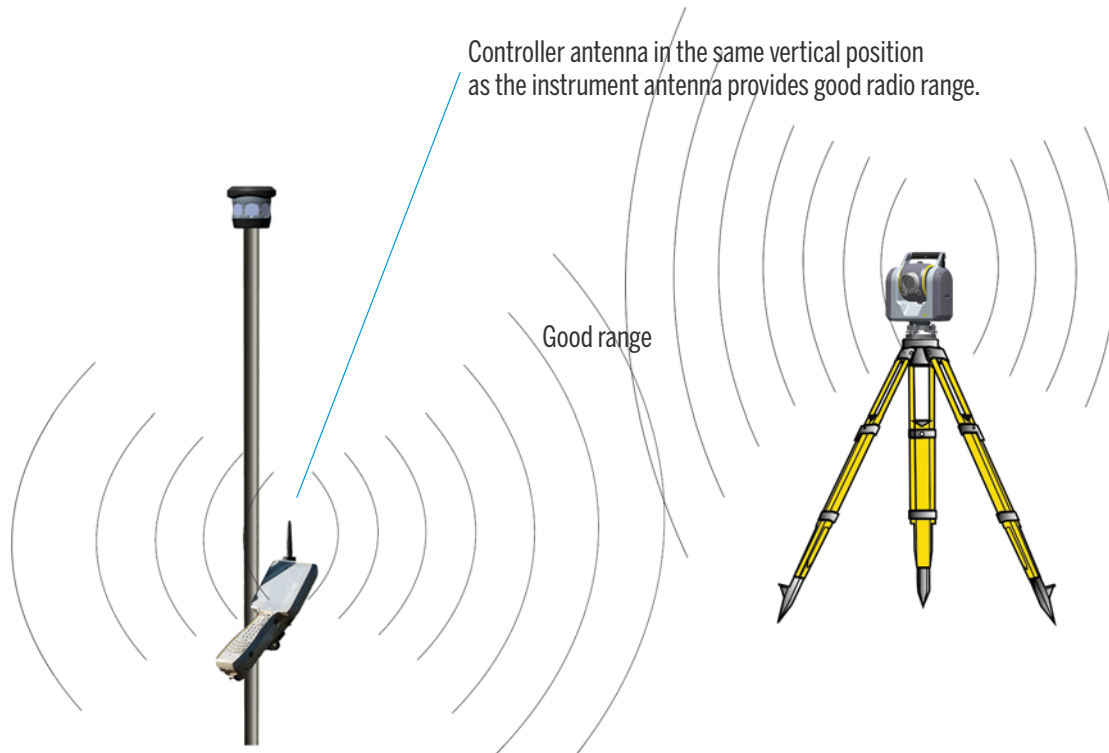
Figure 4.8 Good radio range with controller antenna in the same vertical position as the instrument antenna
